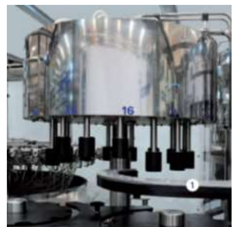
The rotary Turret Deox system uses a high vacuum pump for removing air from the bottles followed by an injection device for flooding the bottle with inert gas.
